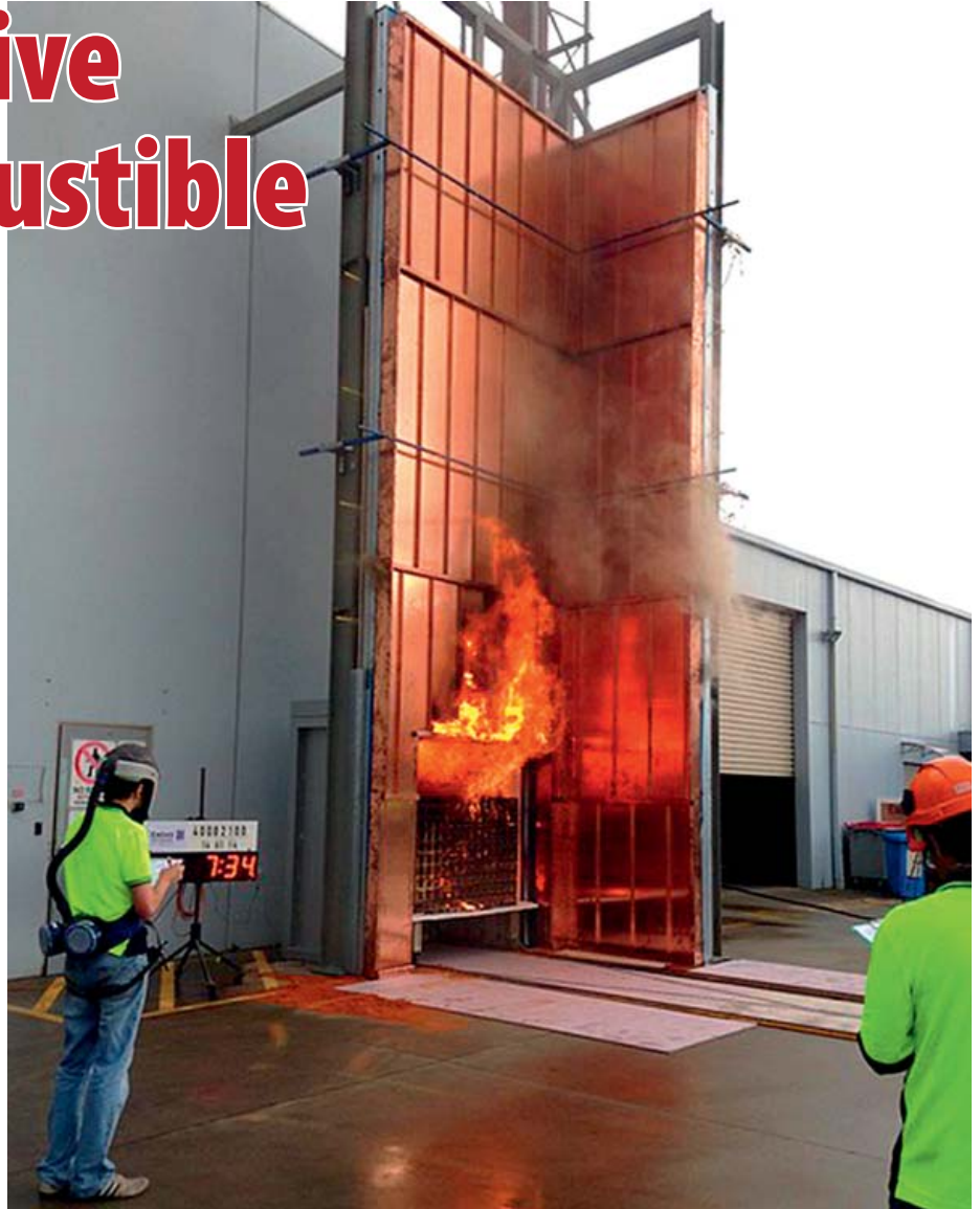
Fire testing the cladding system at the Exova Warrington-fire Aus test facility in Victoria.
